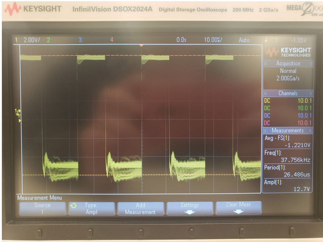
Figure 3.2.3 - Perimeter Wire Emitter Square Wave
